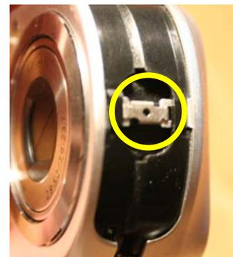
Separate the front and rear halves of the camera, and voila! You are now inside. Set these two pieces off to the side. Take care to set the rear shell down so that dust cannot collect on the inside of the polycarbonate window for the LCD.
