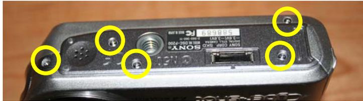
Next, take a small flathead screwdriver as shown below, and pry up on the plastic trim piece that goes the whole way around the camera. This trim piece is not held on by any screws but instead by little plastic clips that protrude from its
