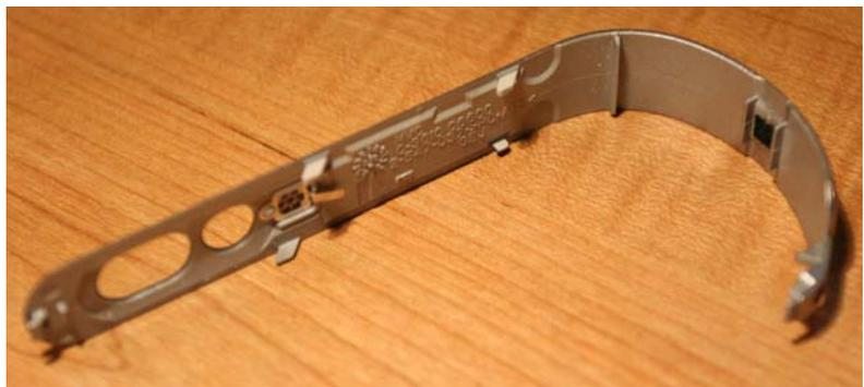
underside (see above). Take care to not damage any of these clips. If you do, that means a call to Sony to replace that trim piece.
